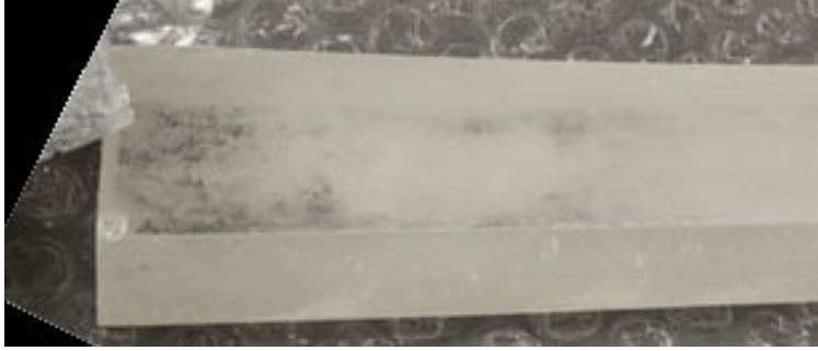
Figure 4.1: Photograph of an OGS scintillator bar being developed into a position-sensitive neutron detector at Saint Mary’s University.
