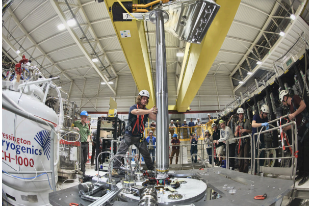
Figure 5.20: The insertion of ALPHA-g anti-hydrogen trap into the ALPHA-g detector at CERN, shown with then UBC student Nathan Evetts.
